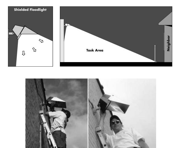
**NOTE** This sheet is intended to describe the best remedy for existing floodlights. For the best performance in new outdoor lighting installations, consider full-cutoff type fixtures instead of floodlights to avoid glare, light trespass, and light pollution.
